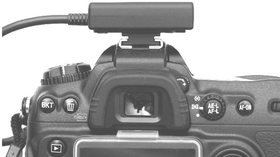
di-GPS USB Mounted on the flash accessory shoe.
