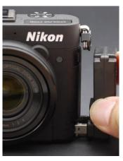
Direct connect Eco PS10-M GPS to the accessory terminal of the DSLR camera body.
